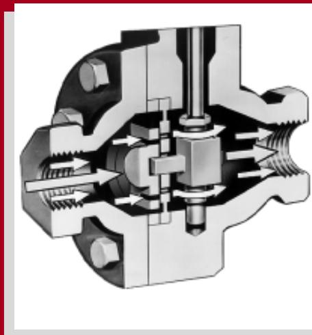
*The straight-through flow path of a sliding gate valve reduces velocity and turbulence and leads to quiet operation and reduced wear.*
